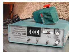
Mobil-FM-Transceiver SE 280, 144-146 MHz in 80 Kanälen
