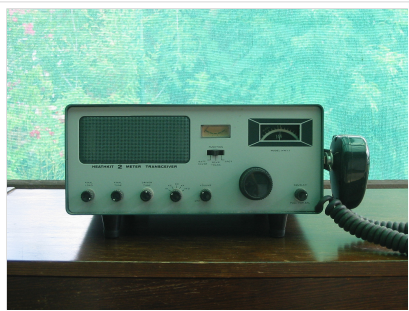
Heathkit HW17 2m AM Transceiver
