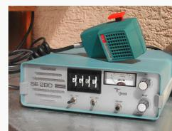
Mobil-FM-Transceiver SE 280, 144-146 MHz in 80 Kanälen
