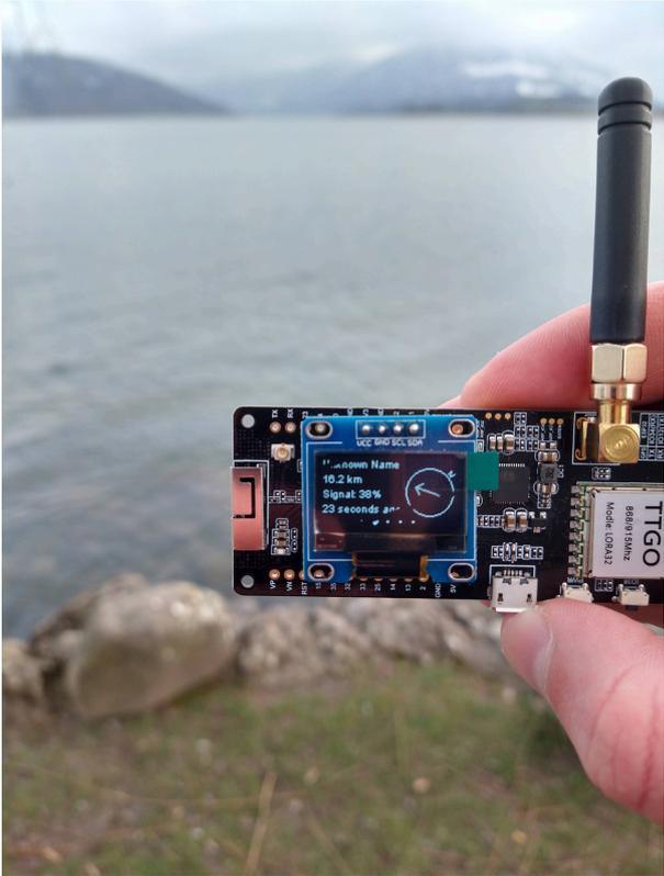
A hand holding a blue LoRa node board with a black antenna. The board has a small LCD screen displaying "Room Name", "10.2 km", "Signal: 38%", and "23 seconds an". The board is labeled "TTGO" and "868/915MHz". The background shows a lake and mountains. |
