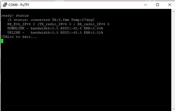
A screenshot of a terminal window titled 'COM9 - PuTTY'. The terminal shows the output of a 'status' command. The text displayed is: 'ready> status', '15 status: connected TA:3.9km Temp:27degC', 'RX Ech IPv4 0 ;TX radio IPv4 0 ; RX radio IPv4 0', 'DOWNLINK - bandwidth:0.0 RSSI:-62.4 ERR:0.00%', 'UPLINK - bandwidth:0.0 RSSI:-65.0 ERR:0.01%', and 'CTRL+c to exit...'. There is a green cursor at the end of the last line. |
