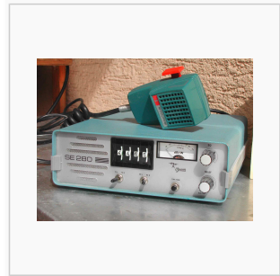
Mobil-FM-Transceiver SE 280, 144-146 MHz in 80 Kanälen
