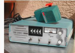
Mobil-FM-Transceiver SE 280, 144-146 MHz in 80 Kanälen
