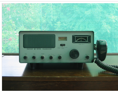
Heathkit HW17 2m AM Transceiver
