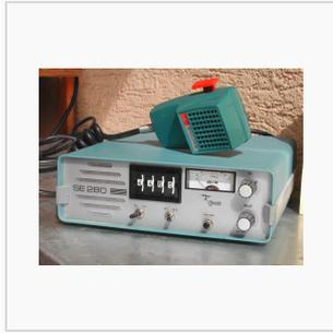
Mobil-FM-Transceiver SE 280, 144-146 MHz in 80 Kanälen
