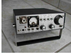
Semcoport 2-m FM /AM Transceiver
