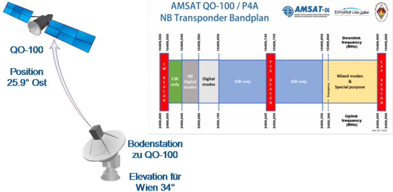
**QO-100 Downlink NB-Transponder** 10,489.500 - 10,490.500 MHz ==> 432.500 - 433.000 MHz
