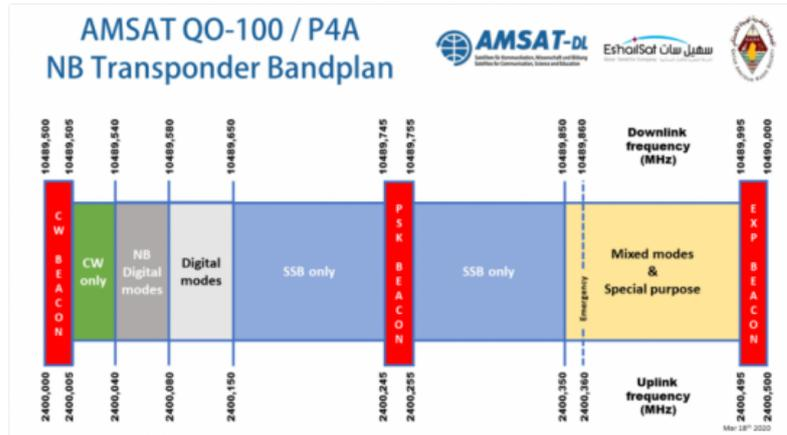
QO-100 Downlink NB-Transponder 10,489.500 - 10,490.500 MHz ==> 432.500 - 433.000 MHz
