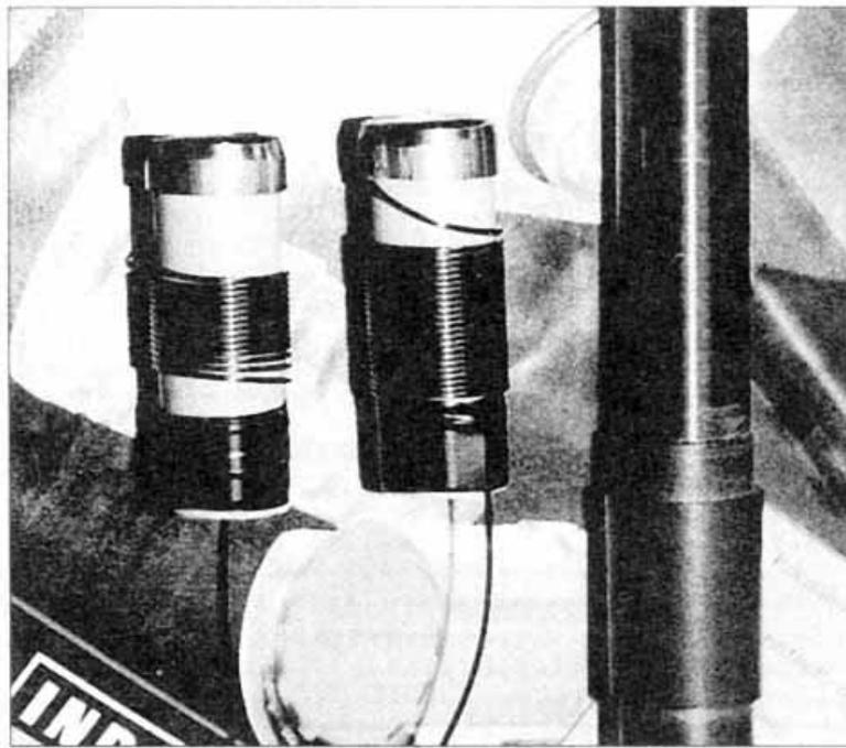
**Fig 6 10m, 20m, 80m inductor coils**
